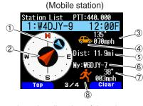
(1) Direction and moving direction of the other station (2) Moving direction of my station
