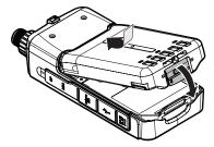
To remove the battery pack, lift the release lever to unlock the battery pack. Lift the battery pack away from the transceiver.
