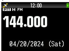
**[Demodulation Mode]:** Displays the demodulation mode.
