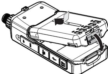
To remove the battery pack, lift the release lever to unlock the battery pack. Lift the battery pack away from the transceiver.
